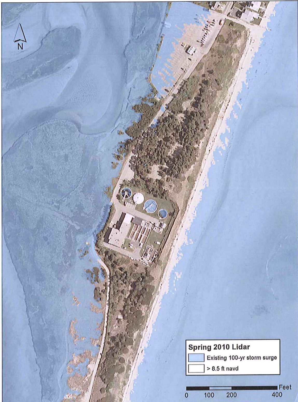
Figure 7. Aerial photograph from 2010 showing the areas that are inundated by flood waters for a 100-year storm event (8.5 feet NAVD) based on existing conditions. The areas shaded in blue would be under water during the storm event. Topographic and bathymetric data utilized for this representation were derived from the 2010 LIDAR survey.
