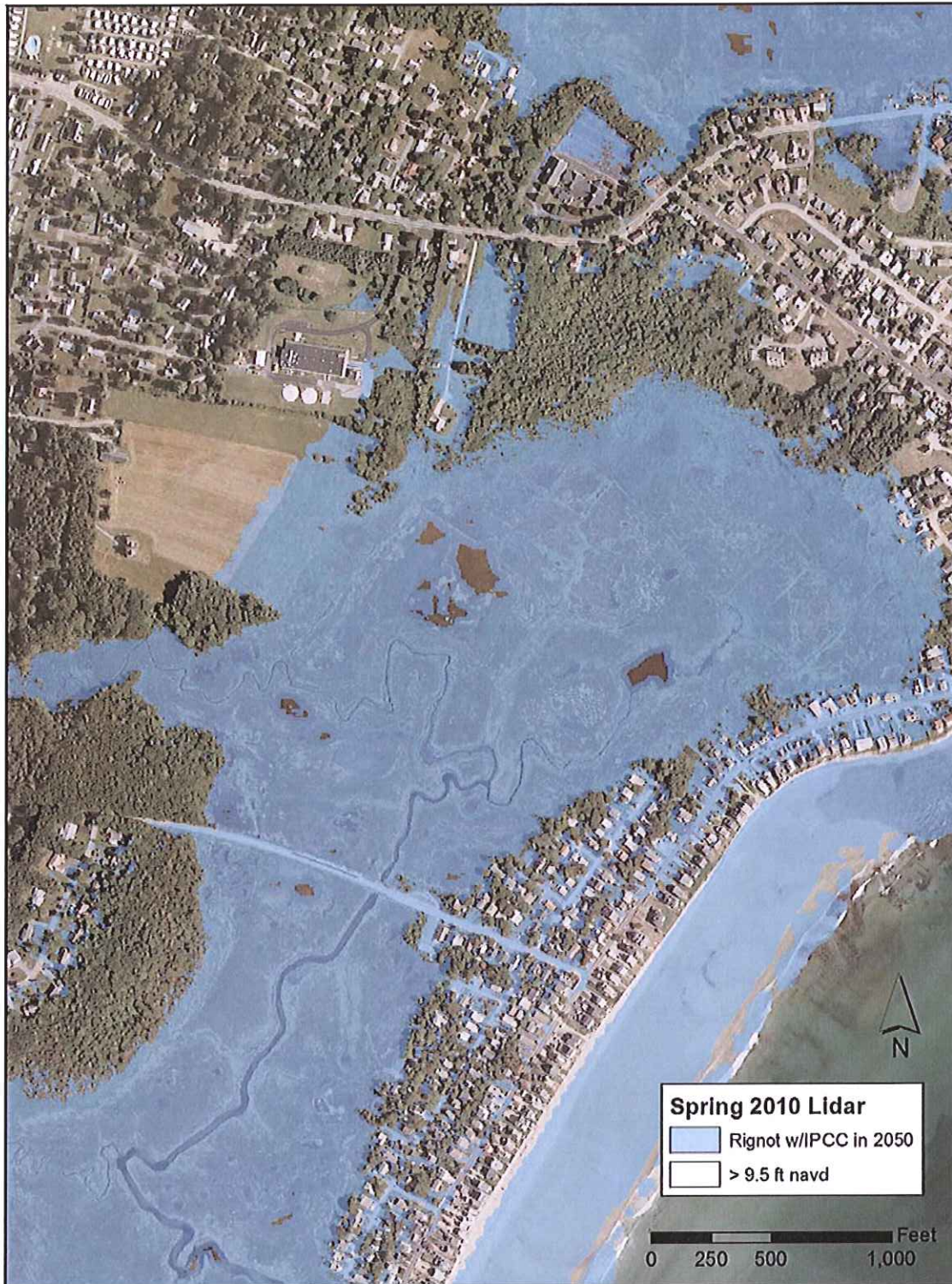
Figure 4. Aerial photograph from 2010 showing the areas that are inundated by flood waters for a 100-year storm event (9.5 feet NAVD) based on IPCC predicted sea-level rise increase in 2050 including updated input for ice sheet contributions (Rignot, et al. , 2011). The areas shaded in blue would be under water during the storm event. Topographic and bathymetric data utilized for this representation were derived from the 2010 LIDAR survey.
