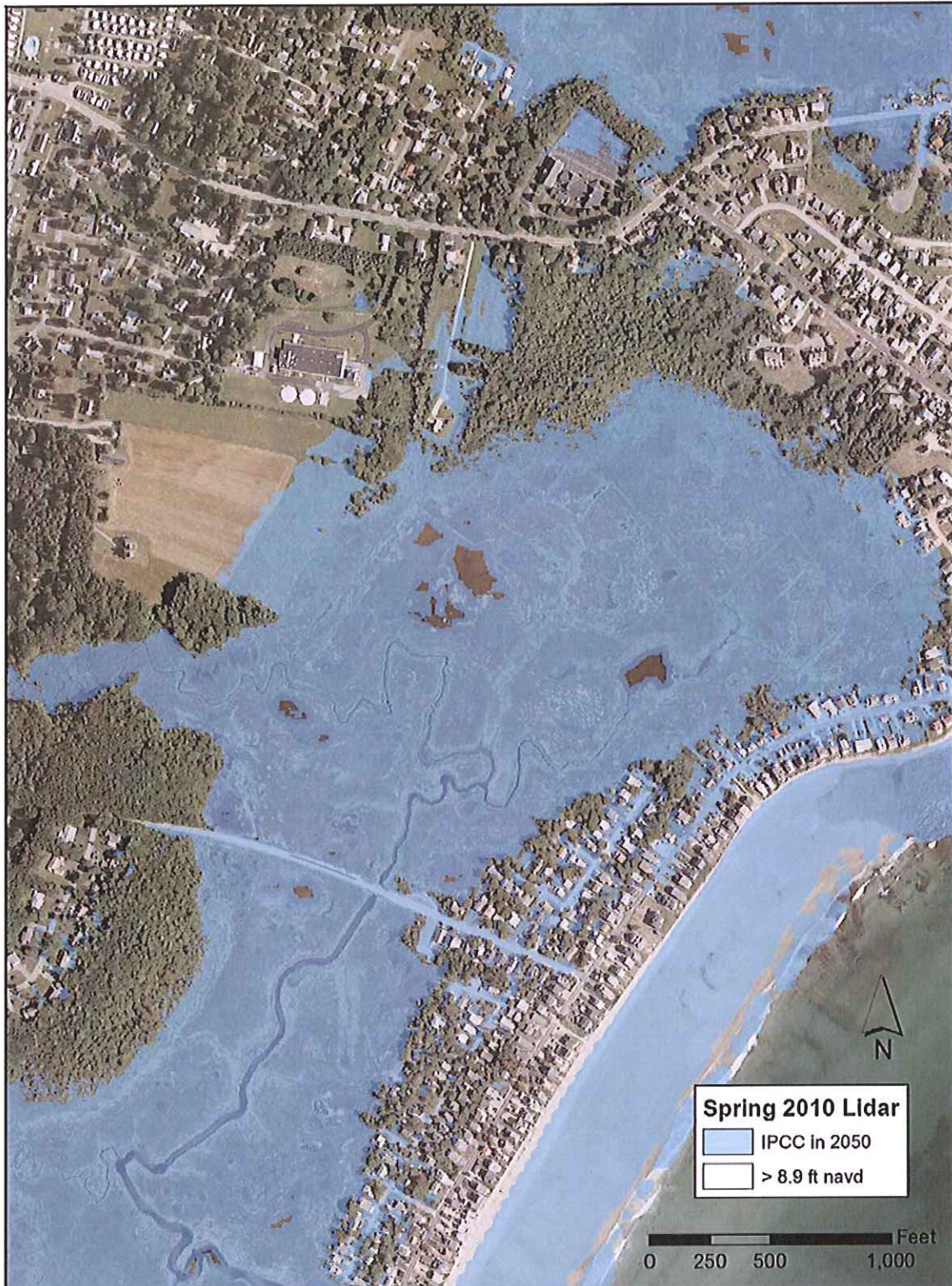
Figure 2. Aerial photograph from 2010 showing the areas that are inundated by flood waters for a 100-year storm event (8.9 feet NAVD) based on IPCC predicted average sea-level rise increase in 2050. The areas shaded in blue would be under water during the storm event. Topographic and bathymetric data utilized for this representation were derived from the 2010 LIDAR survey.
