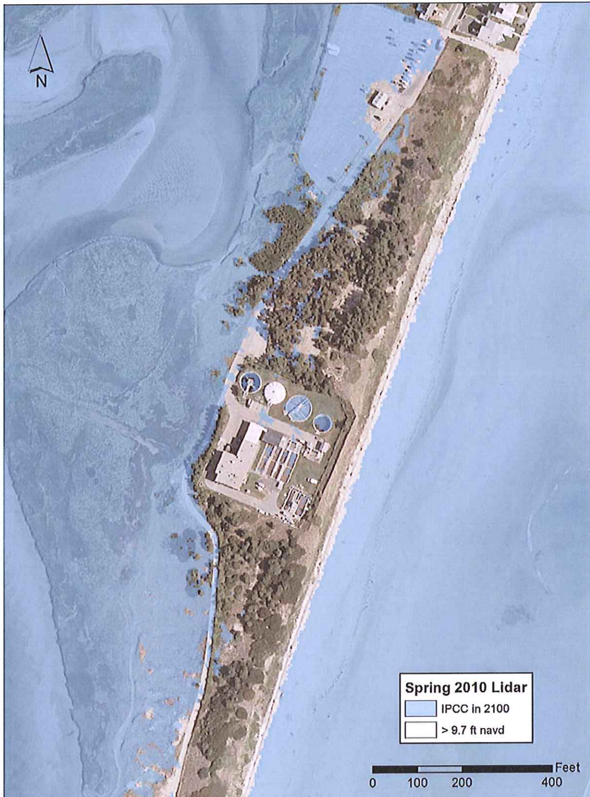
Figure 9. Aerial photograph from 2010 showing the areas that are inundated by flood waters for a 100-year storm event (9.7 feet NAVD) based on IPCC predicted average sea-level rise increase in 2100. The areas shaded in blue would be under water during the storm event. Topographic and bathymetric data utilized for this representation were derived from the 2010 LIDAR survey.
