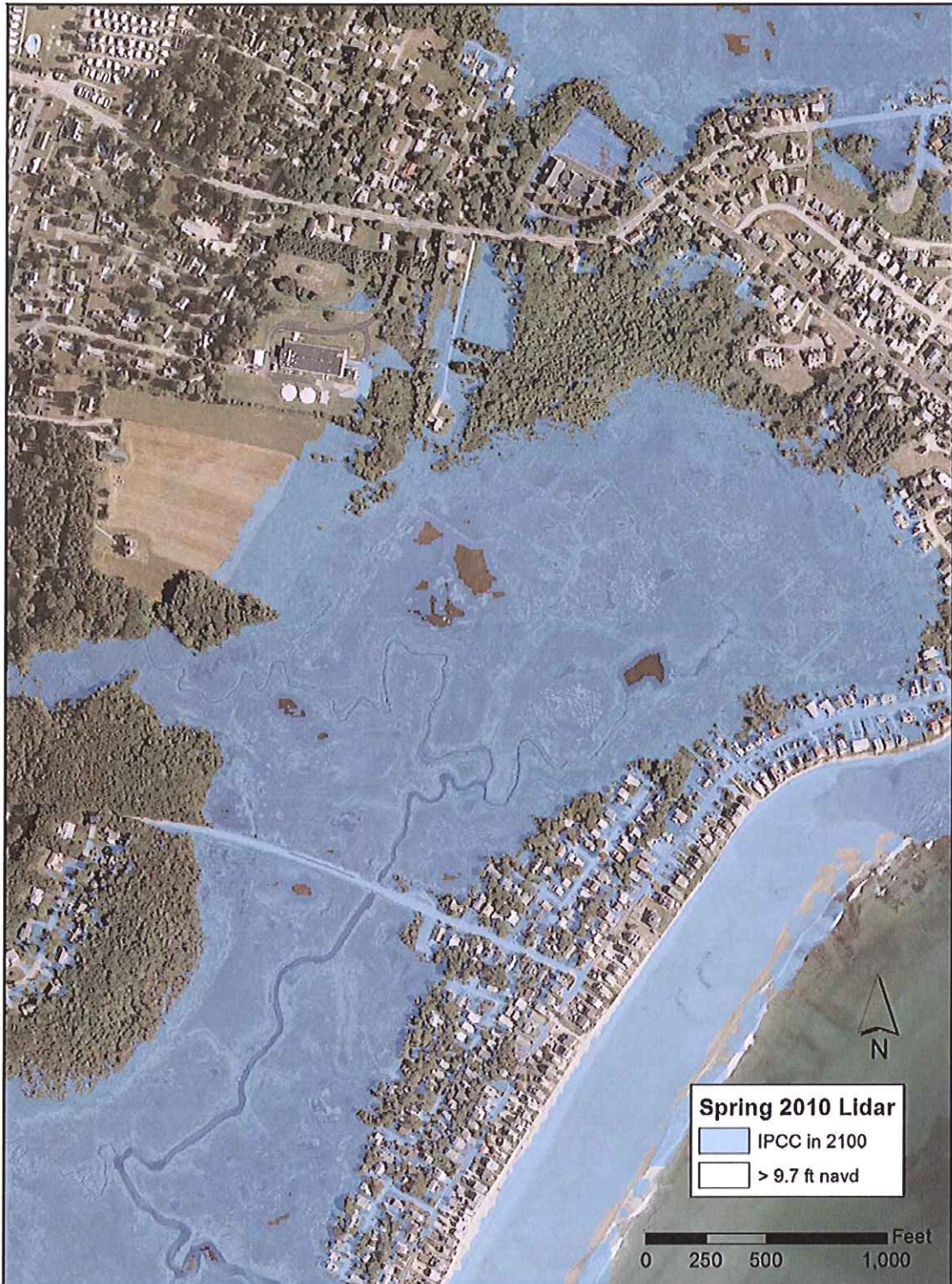
Figure 3. Aerial photograph from 2010 showing the areas that are inundated by flood waters for a 100-year storm event (9.7 feet NAVD) based on IPCC predicted average sea-level rise increase in 2100. The areas shaded in blue would be under water during the storm event. Topographic and bathymetric data utilized for this representation were derived from the 2010 LIDAR survey.
