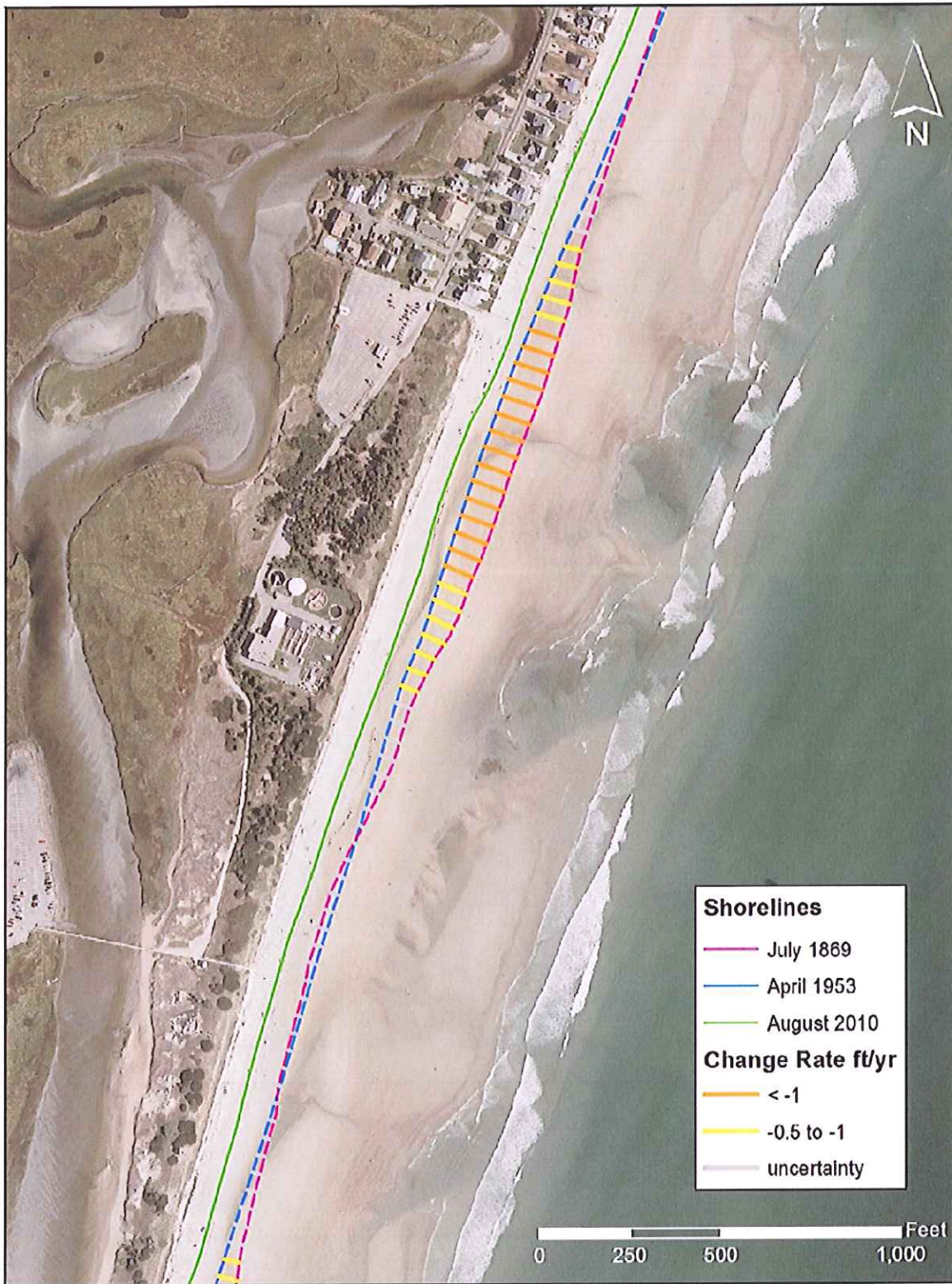
Figure 13. Long-term shoreline change between 1869 and 1953 for the section of Ogunquit Beach fronting the Ogunquit Waste Water Treatment Plant. Shoreline change is color-coded, where the highest erosion rate is represented as orange and areas of minimal shoreline change are represented as grey.
