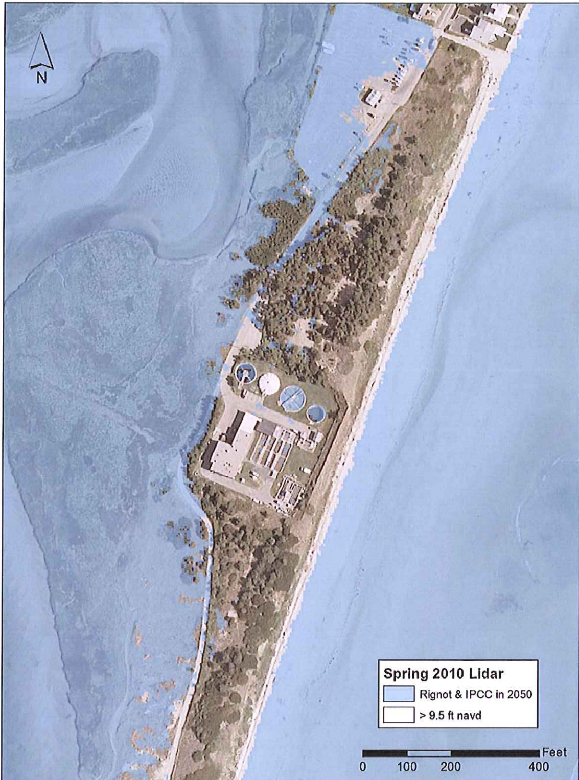
Figure 10. Aerial photograph from 2010 showing the areas that are inundated by flood waters for a 100-year storm event (9.5 feet NAVD) based on IPCC predicted sea-level rise increase in 2050 including updated input for ice sheet contributions (Rignot, et al. , 2011). The areas shaded in blue would be under water during the storm event. Topographic and bathymetric data utilized for this representation were derived from the 2010 LIDAR survey.
